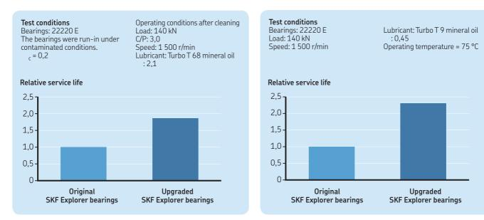
The SKF Engineering & Research Centre performed endurance tests under specific conditions of contamination and poor lubrication to verify performance improvements of the upgraded SKF Explorer bearings.
