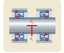
Heavy axial loads and stresses are induced in the bearings system if the non-locating bearing experiences "stick-slip" or is restricted from moving axially.
