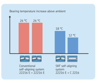
The temperature of the bearings was significantly reduced by the SKF self-aligning system, which includes an SKF spherical roller bearing and a CARB bearing. Reducing the operating temperature extends the relubrication interval
