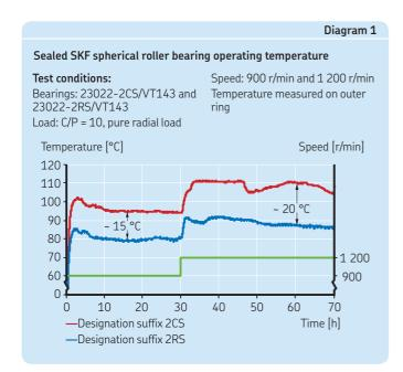
The reduced seal friction of the bearings with improved performance (designation suffix RS) results in lower operating temperature, enabling extended relubrication intervals.
