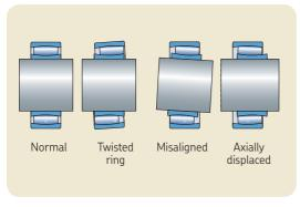
The rollers in a CARB toroidal roller bearing adjust automatically so that the load is distributed evenly along their entire length.
